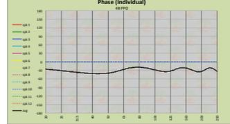
Notice the consistent average phase  $\pm 15^\circ$  for microphones 1 through 7 within the intended bandwidth. Past -6 dB ONAX at 100 Hz pattern breakup causes increasingly irregular average phase.
